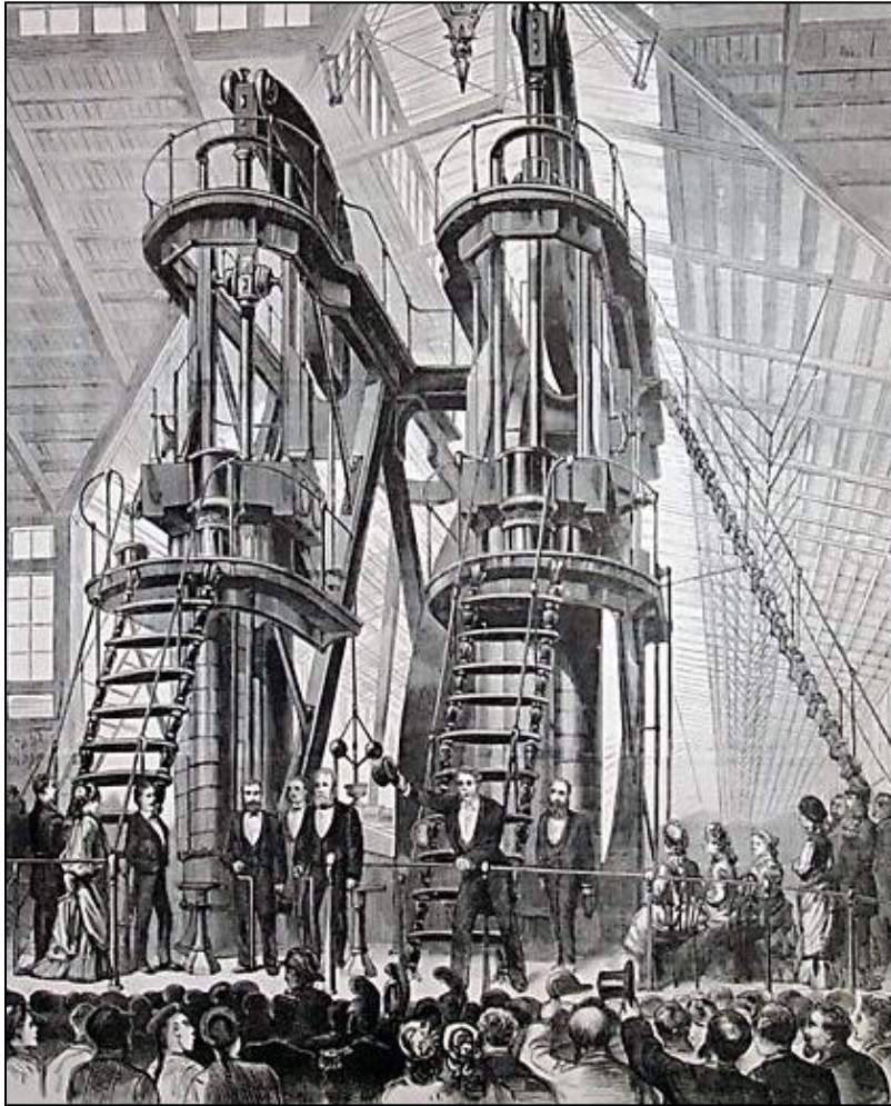
The Corliss Steam Engine, 1876 1,400 horsepower, 40 feet tall, 200+ tons
