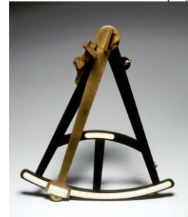
18 th -c. octant similar to that invented by Thomas Godfrey, a Philadelphia optician
