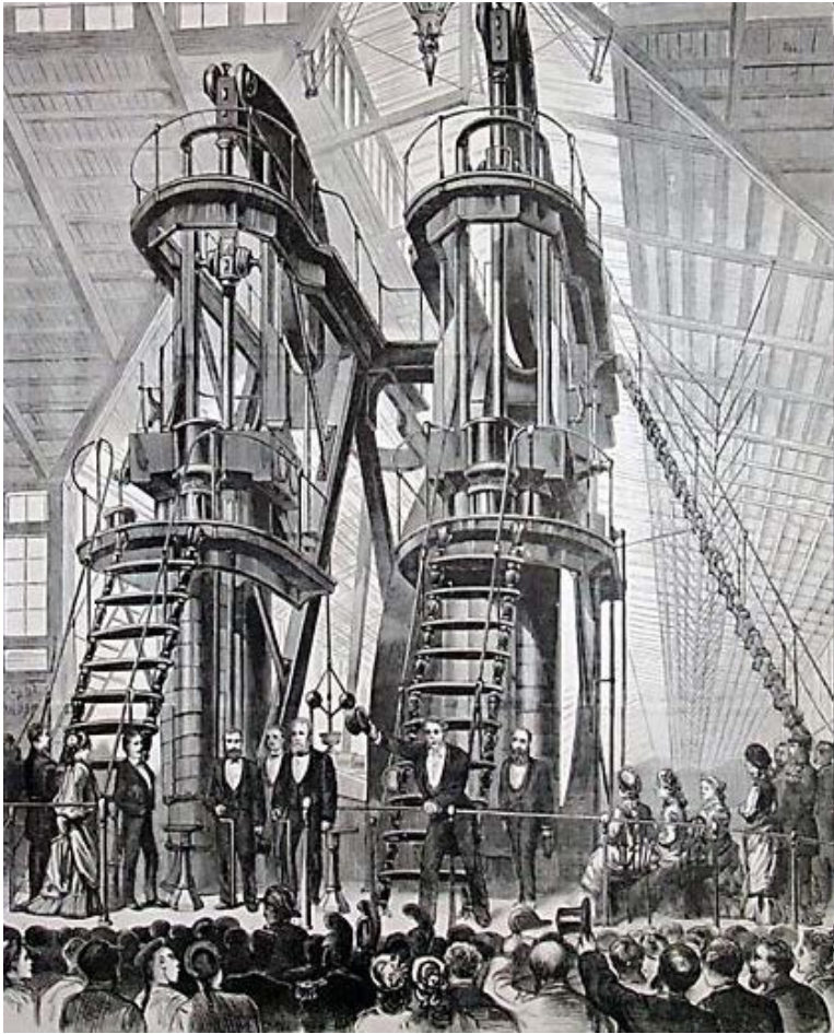
The Corliss Steam Engine 1,400 horsepower, 40 feet tall, 200+ tons
