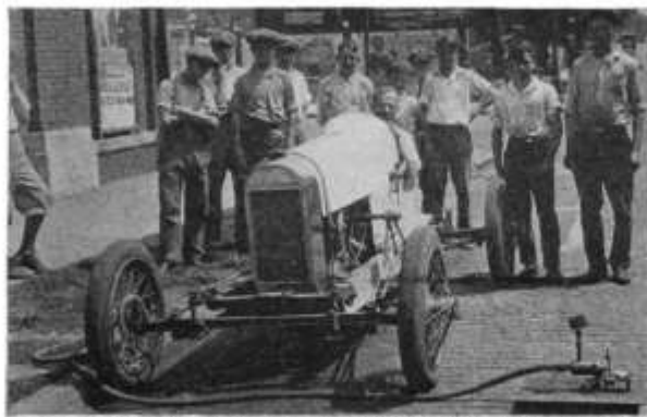
Hydraulic timing device for racing cars depends on the incompressible water in the hose
